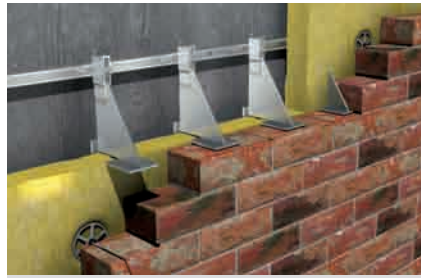
Insulating materials in two-leaf external walls
